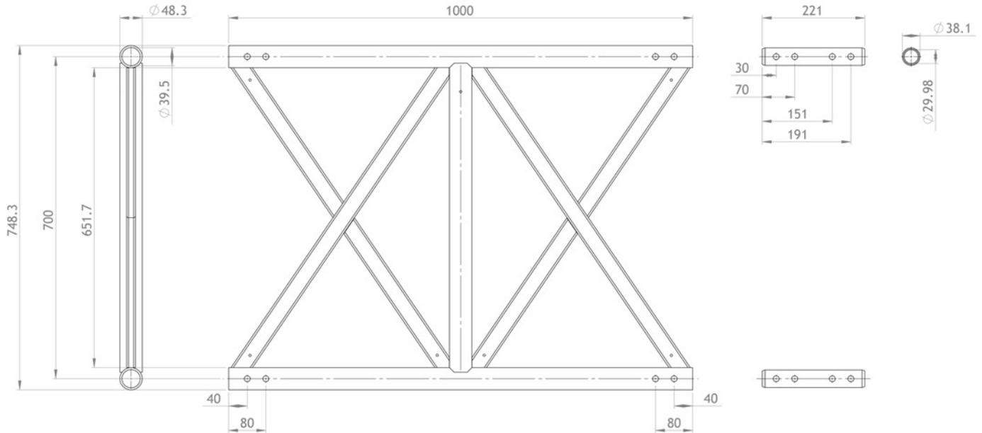
Spigot connections can be introduced at any location in a beam span and don't impact on the beam capacities quoted
